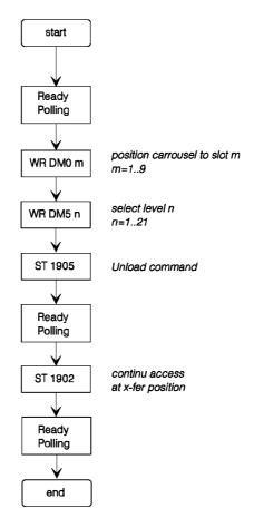
A universally usable procedure which can be used for most StoreX commands is given below. Use this procedure after initializing the instrument only.
