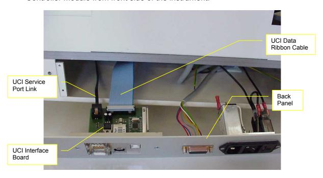
Remove UCI Data Ribbon Cable and pull out Controller Module plate from front side
