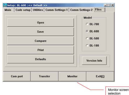
Switch on a monitor mode (button "Monitor").
