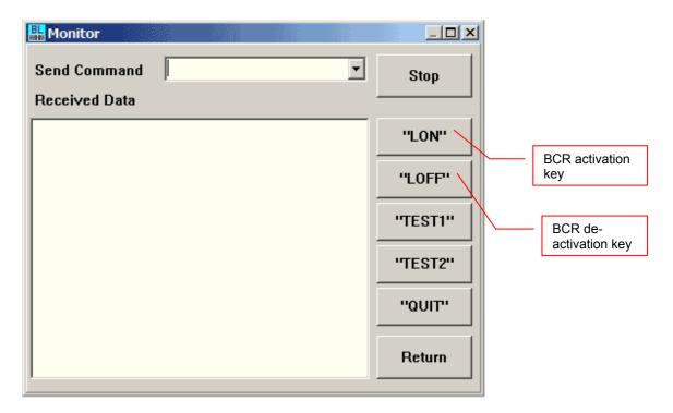
Turn a laser beam on with "LON" button. Please check the beam, is it turned on? Turn a laser beam off with "LOFF" button. Is it "ERROR" string on "Received Data"?
