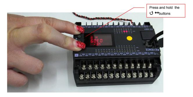
Step 2: - Press and hold **♂** and **⇔** simultaneously - A green flashing test pattern will appear on the display
