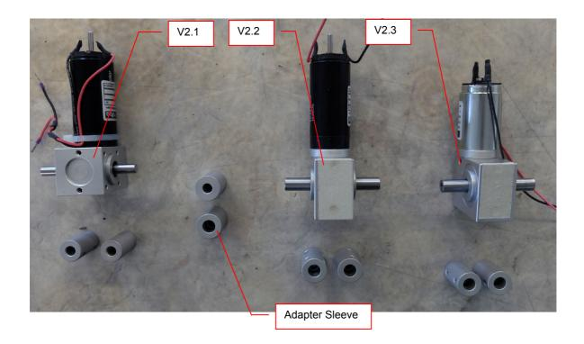
Version 2.2 and V2.3 are interchangeable. To replace a version 2.1 motor-gearbox two Adapter Sleeves are required.
