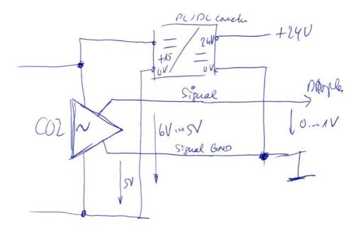
This circuit results in a 0..1V signal voltage at the Display Signal Input instead of the 5..6V of the previous version circuit.
