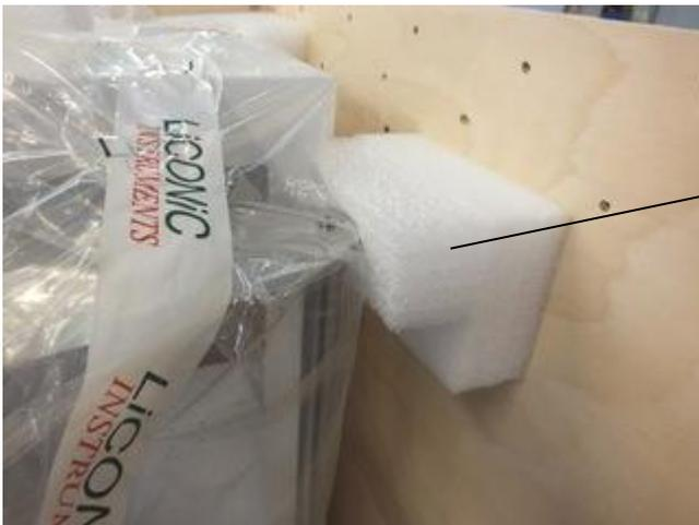
Adjust and glue in the etafon angle to secure the turntable
