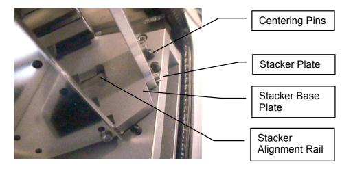
To remove a stacker pull the stacker handle slightly backwards, tilting it, then lift the stacker until it loosens from the stacker alignment rail. Use both hands for this operation. Never use force.
