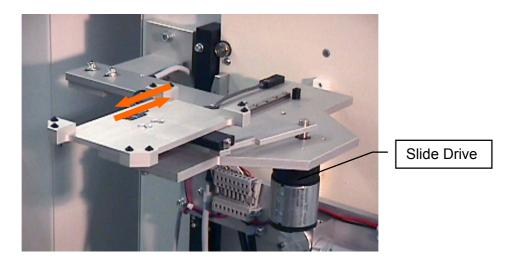
The movements of the Shuttle Station are controlled by the StoreX system. Each time a plate is accessed by the StoreX handling, the Transfer Plate is moved towards the StoreX unit. After access by StoreX the Plate Shuttle is extended towards the external system.
