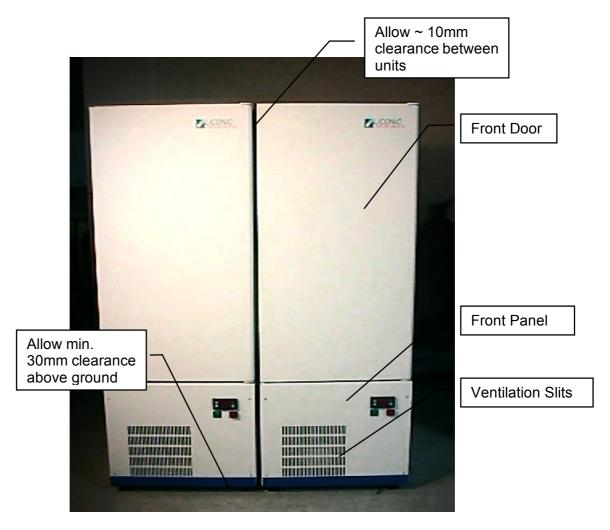
Instruments with cooling options should not be operated immediately after transportation. Leave instrument turned off for at least 12 hours.
