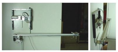
The belt driven system ensures smooth transfer and accuracy of delivery. The Slide Station is normaly in far off Position, when Handler loads or unloads a Plate to the Station the station goes to the load Position.
