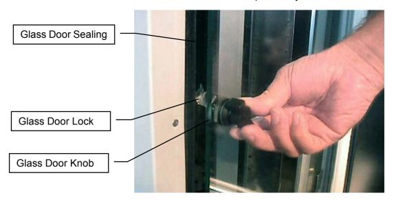
When a Glass Door Access exceeds a certain time period an alarm will sound. This alarm will also prevent the Glass Door from being left open unintentionally. The alarm may be stopped by closing the Glass Door.
