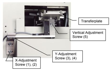
In order to adjust the Transfer Station in the Y-direction (perpendicular to the back-plane) use the screws (3) and (4) and slide the Transfer Sstation into position then tighten screws again. The Height of the Transfer Plate is adjusted by opening screw (5) and lifting or lowering the Transfer Plate. Again, tighten screw (5) after finishing the height adjustment.
