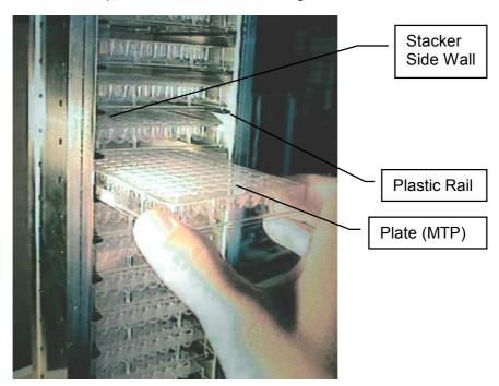
To put a plate in the stacker choose the level and slide the plate along the rails towards the back of the stacker. Slightly lift the front of the plate to avoid excessive wear of the retaining nozzles at the front end of the rails. When the plates are loaded make sure that they are all pushed towards the back of the stacker. Plates that jut out may cause collision with the handler and may result in damage to the handler.
