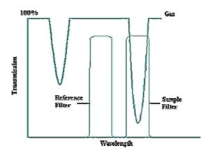
In NDIR gas sensors, an infrared optical 'sample' filter with a narrow band of transmission is selected to overlap with the absorption band of interest, the position of the filter determines which gas will be measured and the amount of absorption determines the gas concentration present.
