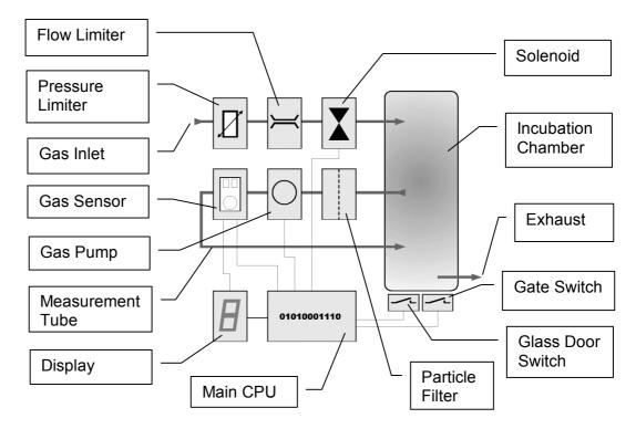
The main CPU monitors the opening of the incubation chamber preventing unwanted gas flow to the surrounding environment. The solenoid is therefore only opened when the glass door is shut and the Gate has not been opened over an excessive period of time.
