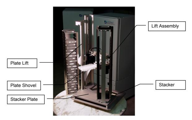
A Handler (4) is used for vertical transport as well as loading and unloading of samples. The Handler consists of a Vertical Positioning Drive (40), a Turn Drive (42) and a Shovel Drive (43). The Handler has a number of vertical positions which are determined by the number of stacker levels and the loading or unloading level.
