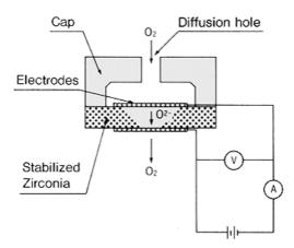
By attaching a cap with an aperture on one side (cathode) of the disc, the gas diffusion is limited and the saturated current is observed. It is termed "limiting current". The limiting current is proportional to the ambient oxygen concentration.
