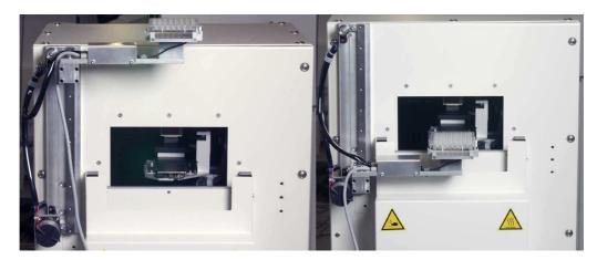
The Lift Station is normaly in upper Position, when Handler loads or unloads a Plate to the Station the station goes to the load Position.
