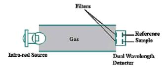
The infrared filter is chosen to ensure that the sensor is totally gas specific and will not exhibit cross sensitivity to other gases.
