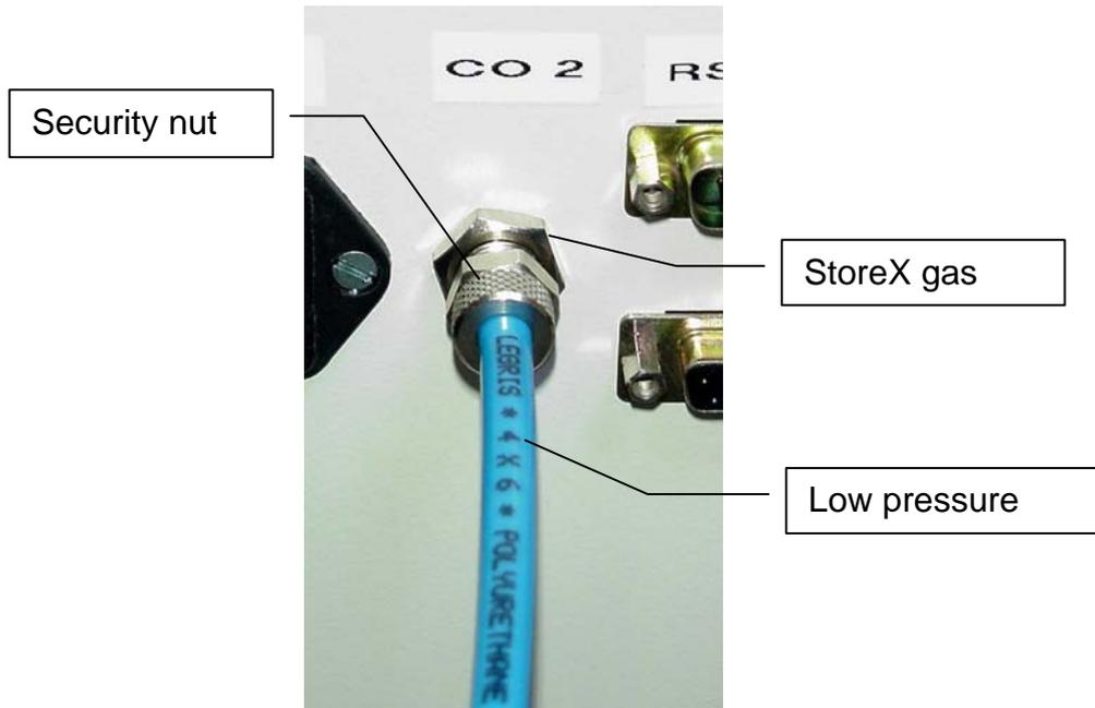
Use 4x6mm PUR, PVC, Neoprene or Nylon tube for the low pressure connection. Do not use Silicon or natural rubber tubing. Make the low pressure tube long enough to allow a minimum of movement of the StoreX for cleaning and maintenance work. For longer length of tubing, copper or other metal tubing should be considered. Foresee flexible tubing next to the instrument.
