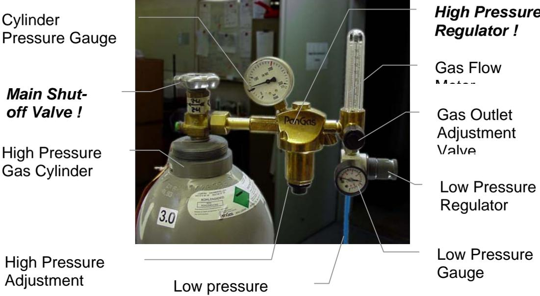
Two-stage pressure regulators are available from gas suppliers or laboratory accessories suppliers. The picture above shows an example of an installation. There is a wide variety of different models available. Your equipment may look different. The gas inlet of the StoreX is located on the back of the instrument. Attach the CO2 low pressure hose securely to the fitting. Always use the security nut. Never operate the unit without the security nut being tightly fit.
