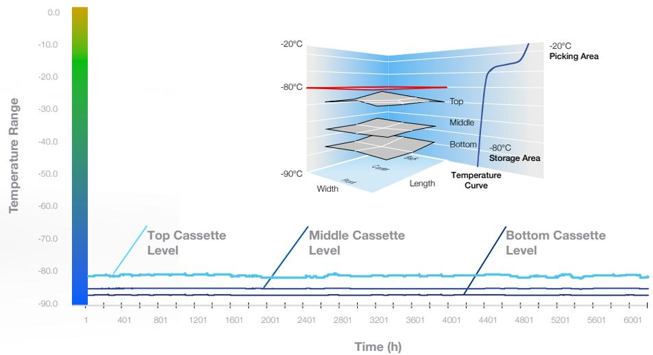
Two climate zones, one for active components at -20°C and another for passive elements at -80°C. Proven, stable horizontal temperature layers within the ULT storage area.
