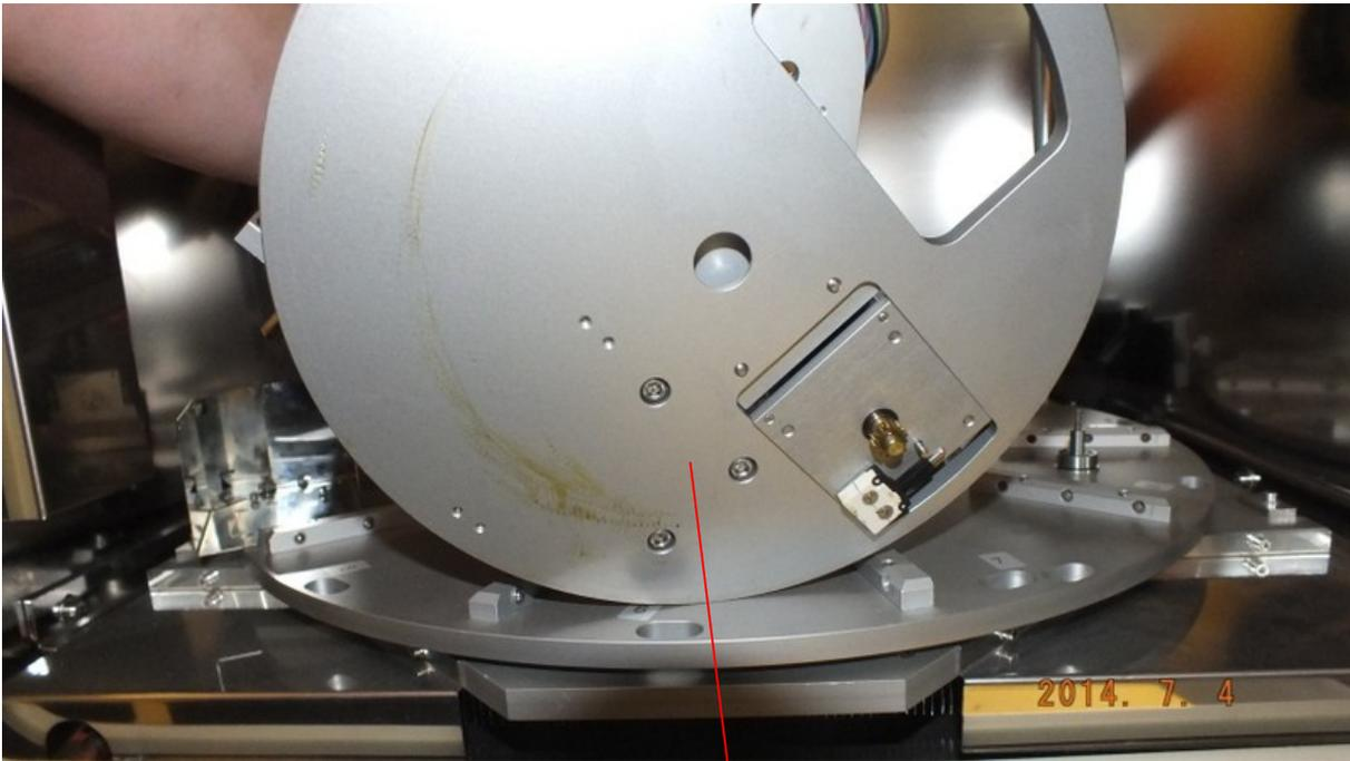
Check these 3 screws if tight, if not tighten and secure with Loctite.
