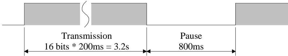
**Figure 3 Overview: Communication Cycle with PLC**
