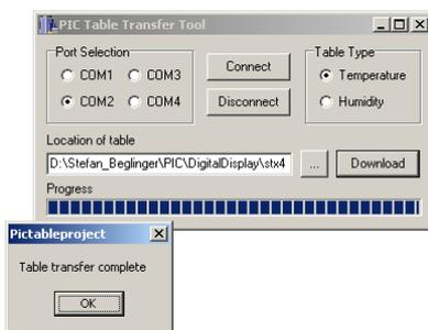
The DDC comes with a user friendly tool to adjust temperature and humidity curve for applications where this is needed. This can be the case if the sensor cannot be placed at a position where it is supposed to be and thus there will be a slight deviation between the actual value and the value from the sensor.
