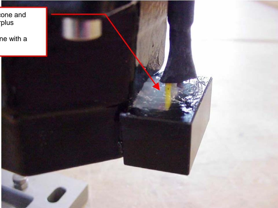
**Picture 5: Finished connector sealing**
