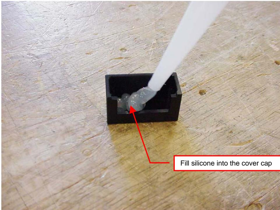
Picture 3: Fill silicone into cover cap
