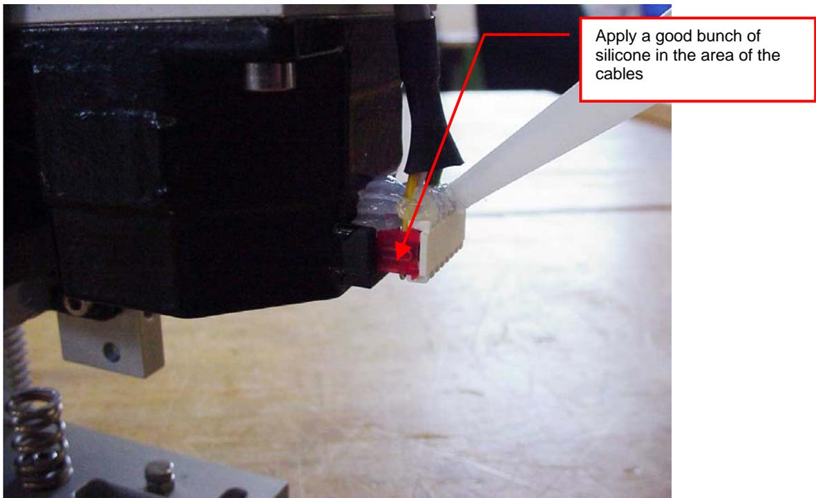
Picture 2: Apply silicone in the are of connectors
