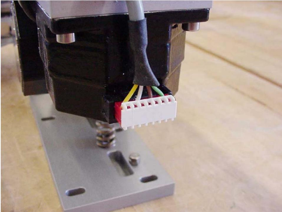
Picture 1: View of connector without any silicone
